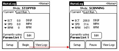
The AutoLog status at the top will change from STOPPED to SCANNING, and will continuously monitor the configured Start parameter & see if it's time to start logging. When the conditions are met, the status will change from SCANNING to LOGGING, and will stay that way until the Stop Logging condition is true, or the max number of seconds is reached.
